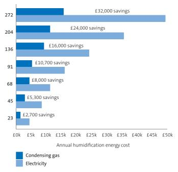
Based on full humidifier output for 2,500 hours per year, gas at 3p/kW and 91% efficiency and electricity at 9p/kW and 94% efficiency.
